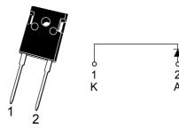
Package:TO-247AC-A ECRP3065A-HF HF=Halogen Free
