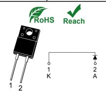
Package:ITO-220AC ECRF465A-HF HF=Halogen Free
